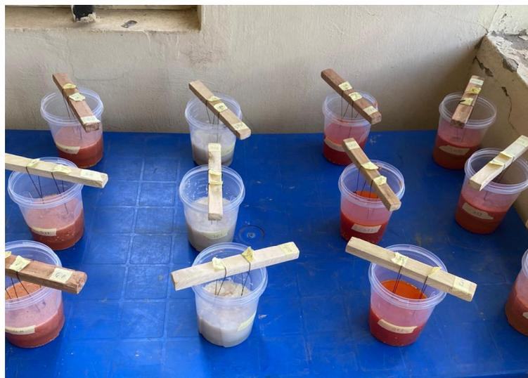
**Fig. 1. Test samples suspended in plastic container containing corrosion test media for 30 days**
